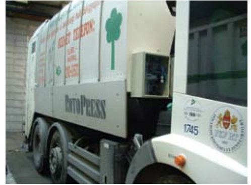
Biothys pneumatic deodorising system on a waste collection vehicle
