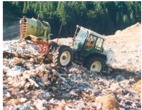
Deodorisation of a waste dump using Biothys technology
